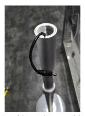
Step 2: Connect the wiring harness interface of the equipment with the wiring of the telescopic rod.
